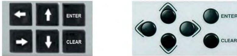
(LEFT) "Square" Button Keypad – Initially Released Chassis (RIGHT) "Round" Button Keypad – Current Production Unit
